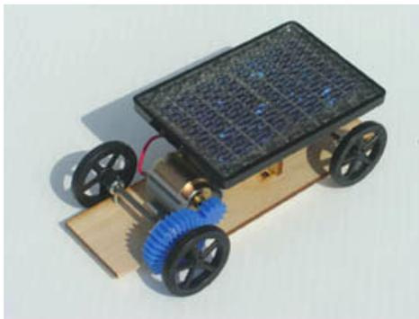
***NOTE:*** *If there is no sunny location outside, you can test the solar powered car with a lamp having strong light (120 Watt) and reflector. Just place the solar car two feet under the strong light for sometimes. Now test the solar car and enjoy the ride.*
